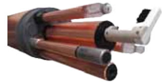
Cleaning of electrodes with wiper
