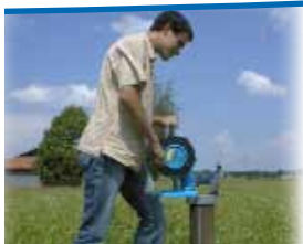
Electric contact meter KLL-Q-2 measuring in ground water
