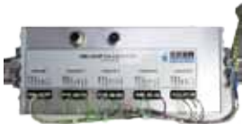
Signal converter RS 485 - 4-20 mA
