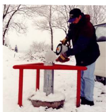
Water level measurement
